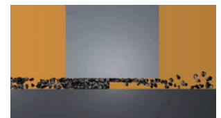
CONTAMINATION IN PRESENCE OF NARROW TOLERANCES
